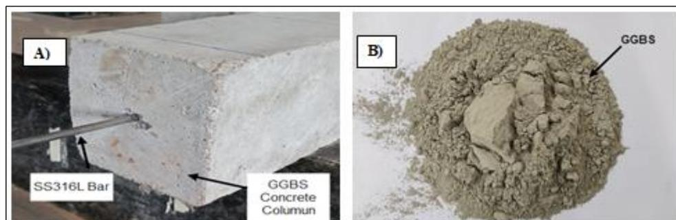
**Figure 1:** A) GGBS Concrete Column Specimen with SS316L and B) Ground Granulated Blast-Furnace Slag (GGBS)
