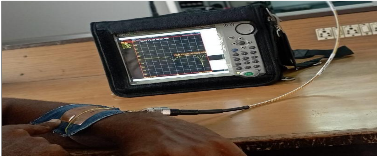
Figure 27: Slight Bending Condition of the Double L-Slot Antenna
