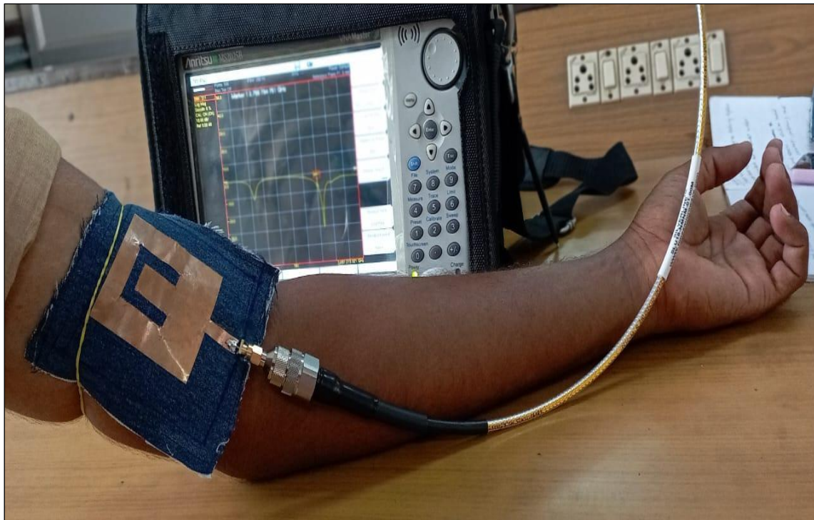
Figure 23: Bending Position of the Inverted U-Slot Antenna
