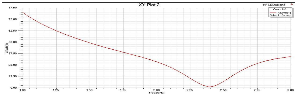
Figure 9: VSWR of Inverted U Slot Patch Antenna
