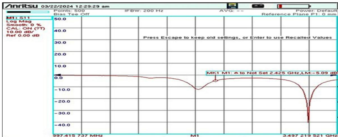
Figure 28: Graphical Output of the Double L-Slot Antenna under Slight Bending Condition
