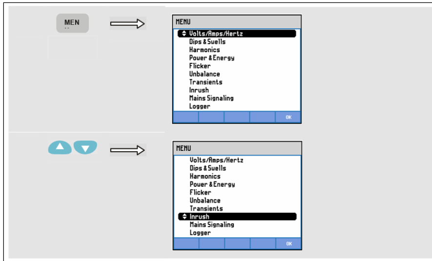
Figure 8: Inrush Current Measurement Setup Menu (20)
